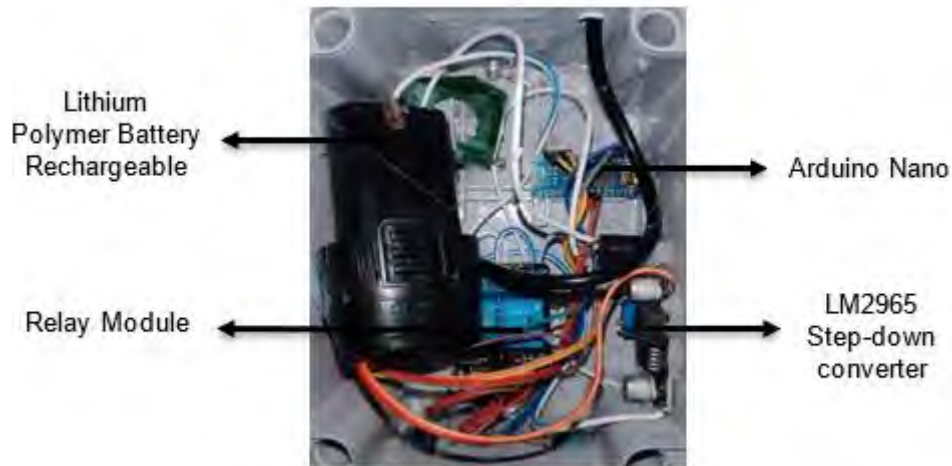
Figure 10: The installation components parts
