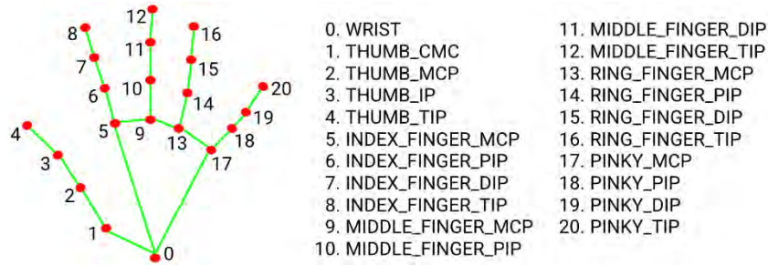
Figure 3: The key landmarks of the hand by Mediapipe Hand Recognition Model
