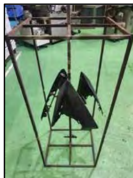
Figure 3.2: New design of sub hanger of Mole 1
