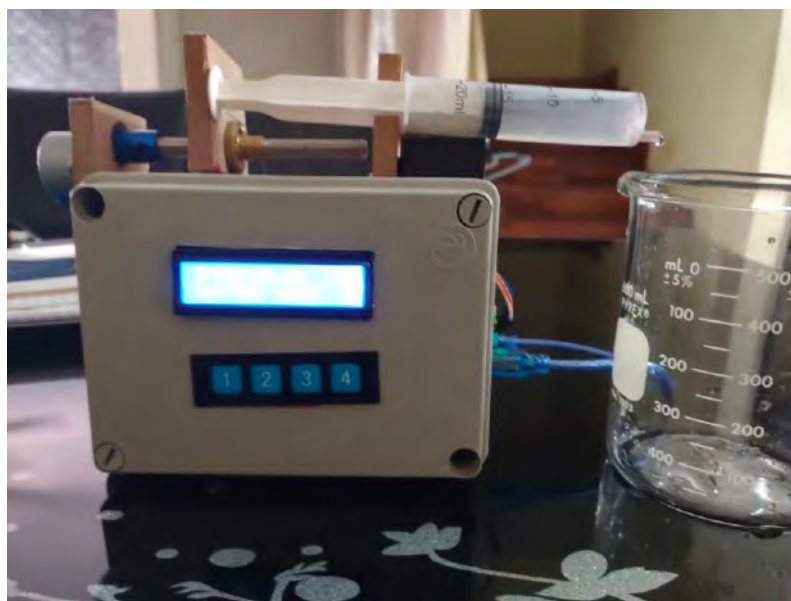
Figure 6: Experiment setting for fluid flow evaluation
