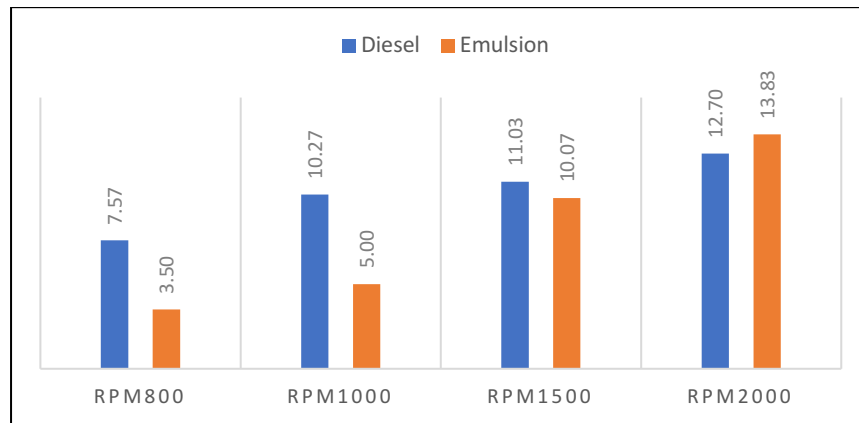
Figure 11: The comparison of smoke opacity between diesel fuel and emulsion fuel under the vehicle's operating conditions ranging from 800 to 1200 rpm
